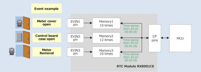
Figure 1 Example of tamper detect function
