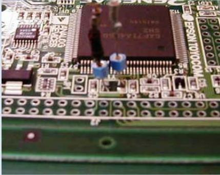
Fig. 2: A resistor is added to measure negative resistance
