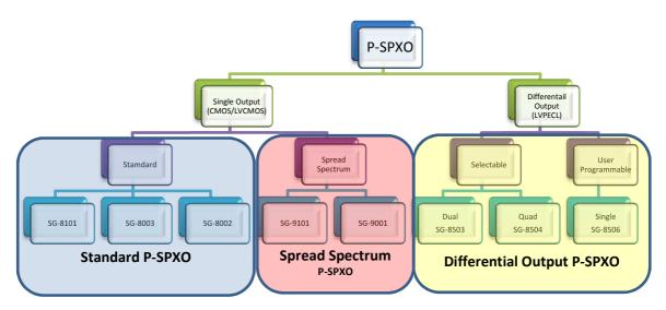
Epson provides standard CMOS output as well as differential output LVPECL. In addition, Epson has series of spread spectrum programmable SPXO to help improve EMI/EMC. Each of Epson's programmable blanks can be programmed with our SG-Writer-II programming tool and appropriate IC adaptors for quick turn prototypes or production builds.
