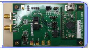
Evaluation Board for User Programmable Devices (I<sup>2</sup>C Interface)
