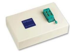
To support rapid product development, Epson's programmable oscillators can be ordered quick delivery from distributors or you can program blanks yourself using Epson's SG-Writer II.
