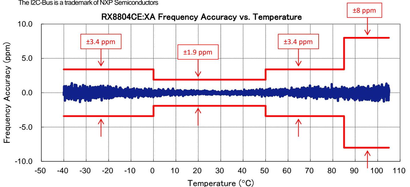
Designed for precision time keeping, Epson's RX8804CE uses Digitally Temperature-Compensated Crystal Oscillator (DTCXO) technology to achieve  $\pm 3.4$  or  $\pm 8$  ppm accuracy over temperature of -40 to +85 °C or -40 to +105 °C respectively, equivalent to  $\pm 9$  or  $\pm 20$  seconds per month. Compared to RTCs integrated into microcontrollers (MCUs), Epson's RX8804CE includes an integrated crystal, is lower power, and is far more accurate.
