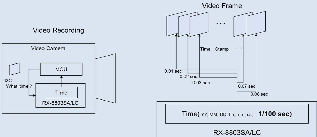
**Figure 4 RX-8803SA/LC 1/100 second data for video frame**
