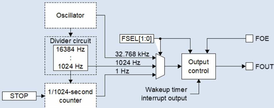
**Figure 1 RA8000CE divider circuit**
