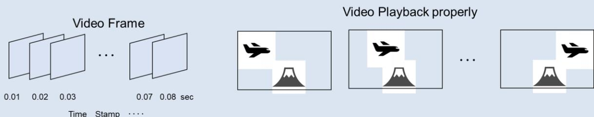
**Figure 5 Proper video playback by 1/100 second timestamp**
