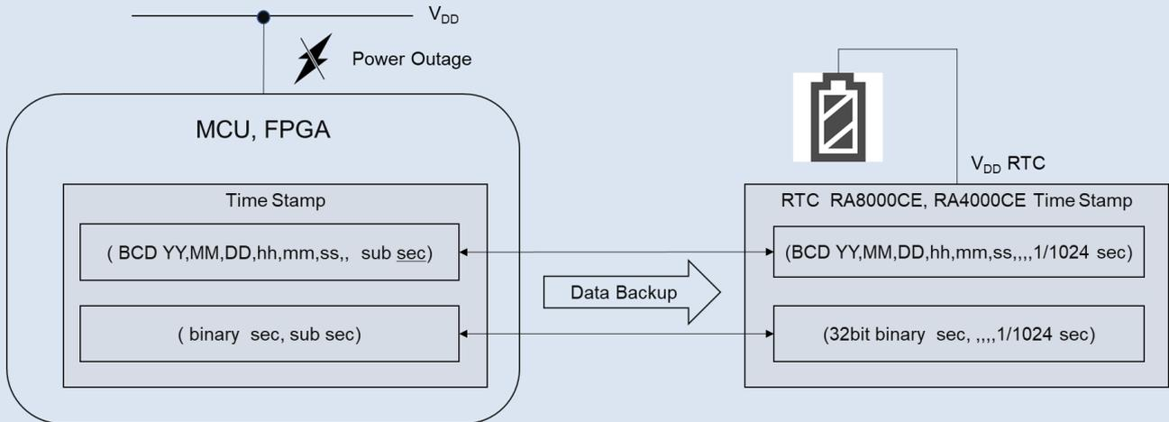
**Figure 8 RA8000CE time stamp backup for MCU, FPGA system**
