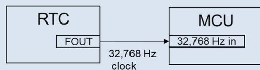
**Figure 3 32768 Hz MCU system clock**
