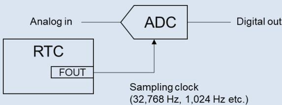
**Figure 2 ADC sampling clock**
