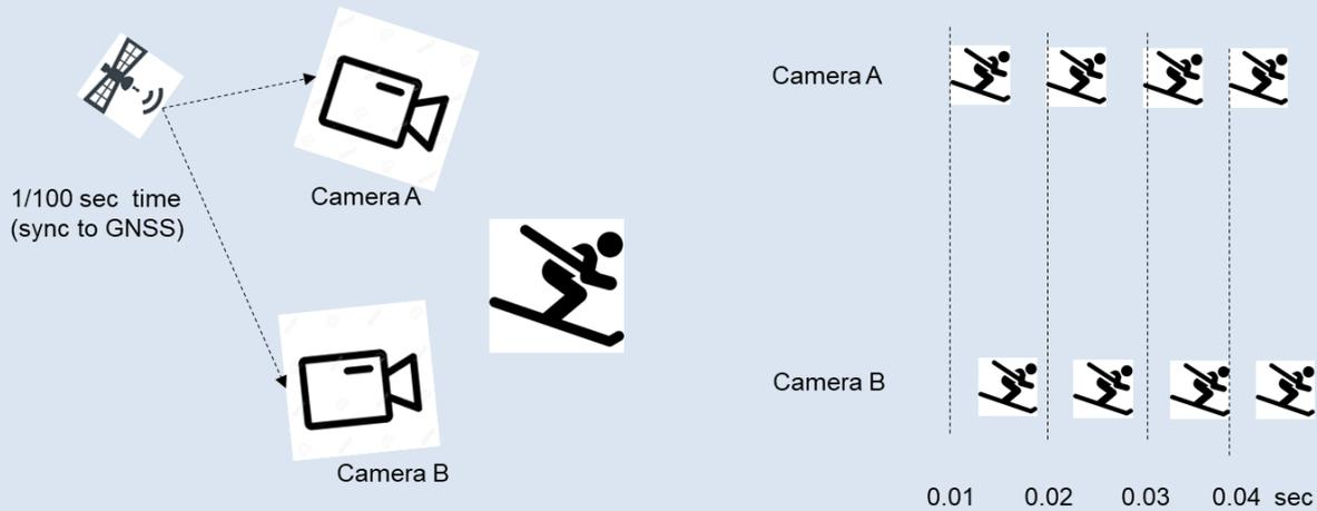
Figure 6 Camera A,B independent 1/100 second time capture
