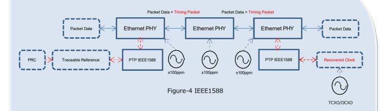
IEEE1588 (Figure 4) transmits frequency and time information from PRTC to target Node by protocol layer. (Basically PTP: Precision Timing Protocol) The target Node has the same time and frequency. This is timing synchronization. All Nodes may be equipped with normal Ethernet Clock. The final Node should be equipped with high stability oscillators. (ex. TCXO, OCXO) to reduce PDV and provide redundant function (backup clock during timing signal interruption.).
