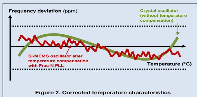
The characteristic shown in brown in Figure 2 is the characteristic after temperature compensation has been applied by Frac-N PLL.
