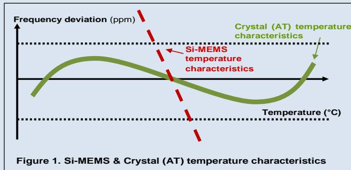
In contrast, silicon resonator temperature characteristics exhibit first-order linearity of -20 to -30 ppm/°C. When an oscillator is constructed using a resonator with these characteristics, the natural temperature characteristics of the crystal have to be compensated. Since crystal units are individually tuned to the desired frequency, initial deviation also shows a ppm-order width of variation.
