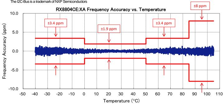
Designed for precision time keeping, Epson's RX8804CE uses Digitally Temperature-Compensated Crystal Oscillator (DTCXO) technology to achieve ±3.4 or ±8 ppm accuracy over temperature of -40 to +85 °C or -40 to +105 °C respectively, equivalent to ±9 or ±20 seconds per month. Compared to RTCs integrated into microcontrollers (MCUs), Epson's RX8804CE includes an integrated crystal, is lower power, and is far more accurate.
